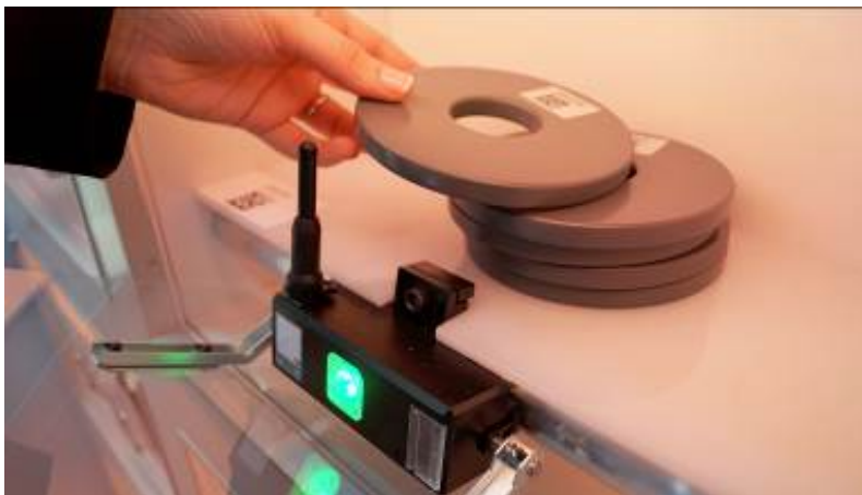
Picture 2: With Mitsubishi Electric Guided Operator Solutions in place, the automation system guides an operator to the correct parts bin, either by lighting an indicator next to the correct picking location or by opening a door. Picks can also be confirmed manually using a touch switch or light curtain.
