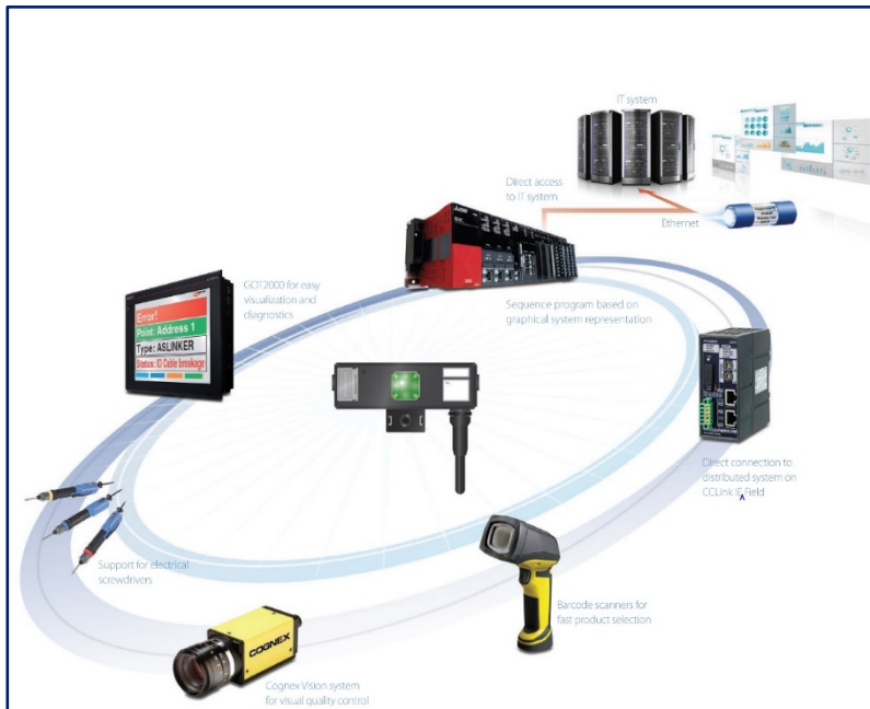
Picture 5: Using advanced control systems also means that manual workstations can be connected to factory wide automation networks and MES systems. This allows greater system transparency and direct access to resource planning systems.
