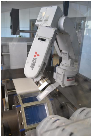
Image 2: It is possible to further improve productivity on the factory floor as well as maintaining a controlled environment in the cleanroom more easily by adding a robotic arm for loading.
