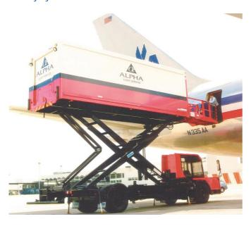
The FX PLCs control each stage of the operation including all the safety interlocks. These prevent the lifts from operating until the vehicle is stable on the hydraulic rams and uses high-speed limit switches to prevent the lifts from over reaching, so avoiding potential damage to aircraft. Their integral Real-time clocks (even on the smallest PLC) enable Norquip to use real-time switching on vehicle enunciators, allowing them to meet local noise restrictions regulations.
